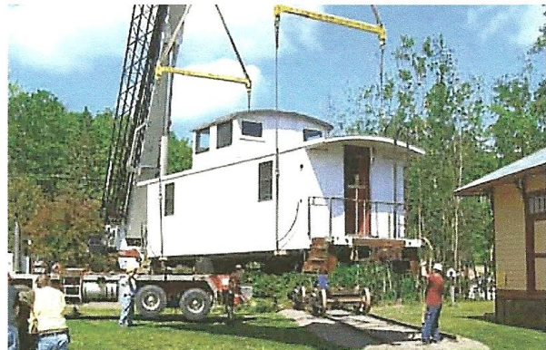
Above Left: Soo caboose no. 593 was staged in a parking area next to the National Railroad Museum in Green Bay on June 2, 2009. Above Right: One of AZCO's mobile cranes prepares to lift the 593 off its trucks. Notice how the crane's outriggers have been placed to stabilize it. Bottom Left: The 593 has been loaded onto a low-boy trailer and is being prepared for its trip to Stone Lake. To get the 593 under one low bridge, the driver had to stop and let the air out of each of trailer's tires. Bottom Right: In its new home, the 593 is being placed back on its trucks next to the restored Soo Line Stone Lake Depot—all photos by Carol McDonnell.
