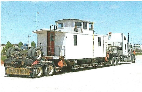
Above Left: Soo caboose no. 593 was staged in a parking area next to the National Railroad Museum in Green Bay on June 2, 2009. Above Right: One of AZCO's mobile cranes prepares to lift the 593 off its trucks. Notice how the crane's outriggers have been placed to stabilize it. Bottom Left: The 593 has been loaded onto a low-boy trailer and is being prepared for its trip to Stone Lake. To get the 593 under one low bridge, the driver had to stop and let the air out of each of trailer's tires. Bottom Right: In its new home, the 593 is being placed back on its trucks next to the restored Soo Line Stone Lake Depot—all photos by Carol McDonnell.
